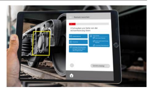
carry out the work steps. The AR application also displays the installation positions, measured values, limit values or circuit diagrams of the components to be processed. In this way, augmented reality helps to increase the reliability of service and maintenance processes and reduce the risk of errors.
