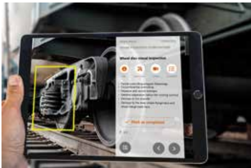
Fig. 1: AR application on the tablet shows the correct position of the work step to be performed. Photo: ZEDAS GmbH
