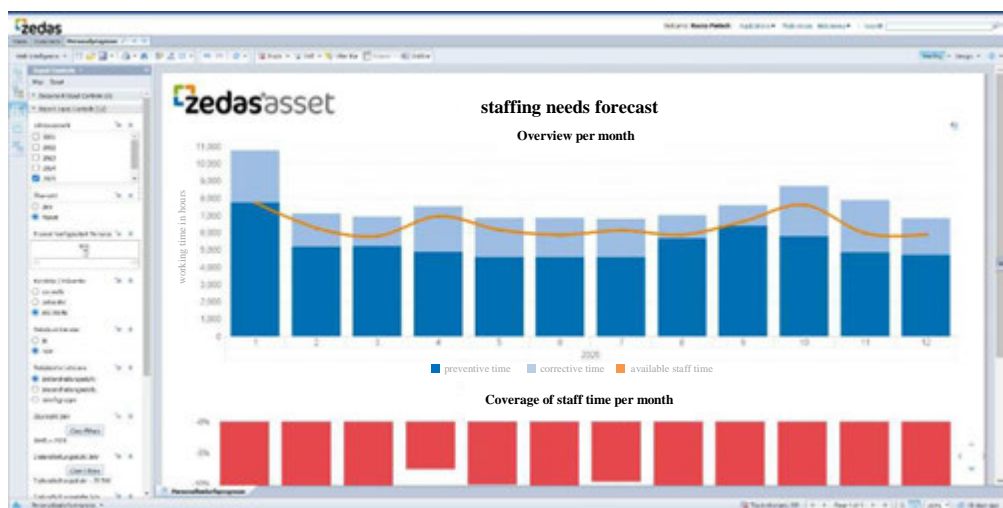
The dashboard shows the ratio of preventive and corrective maintenance actions to staff availability
