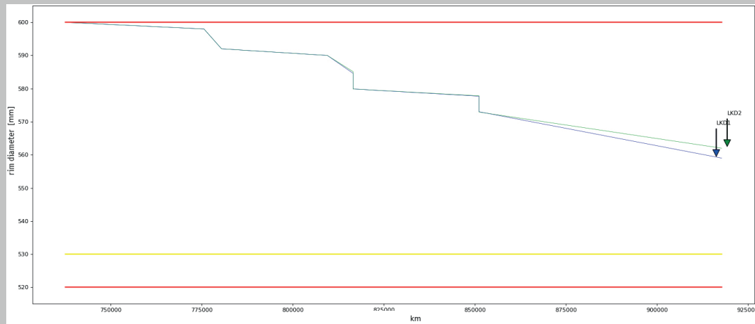
2: Typical measurement data curve for the tread diameter of the two wheels on a wheelset with warning threshold and limit values incl. typical reprofiling jumps
