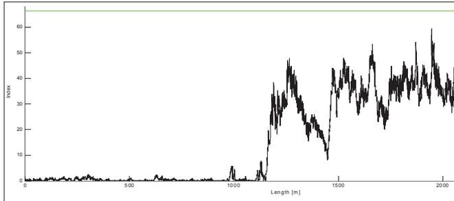
Fig. 14: Evaluation of change in track condition with change with multi-variate index and limit value
